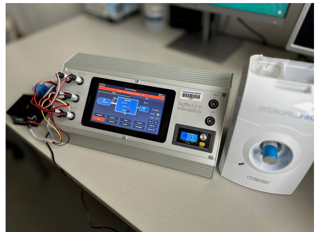
Fig. 2. Required equipment for lab exercises. left: H2-Engineering Kit with proton exchange membrane; right: HydroFill Pro with inserted Hydrostik [11]
